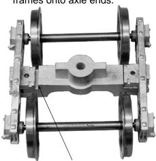
Note gap on stretcher when using Slater's wheelsets. My preferred solution is to reduce axle width by filing off the pin points (plus a couple of strokes) with a flat file.
