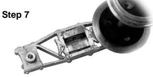
Offer up wheelset to check clearance. Make adjustments as required (possibly chamfer brake block rear with knife blade). When happy solder solid & clean up. Ensure rebate for stretcher end is clean & clear.
