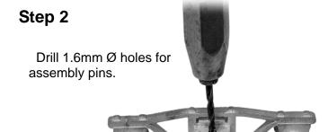
Drill & break through from top and then bottom. Then gently run drill right through to align both holes.
